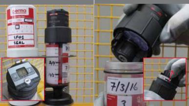
Exchange lubricant canister and battery set.
