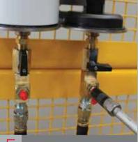
Press the SET button for 1 second to turn lubricator off. Press for another second to turn back on.
