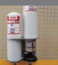
Confirm status using the display screen / flashing lights. The time setting on the display and a green light indicates normal operation.
